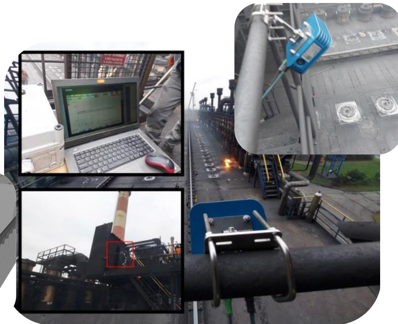
Up to three KY-RAY radar units to watch the scene
